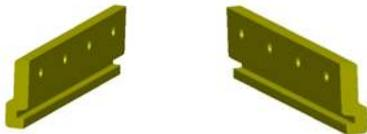
Figure 8. Rail joint plate
