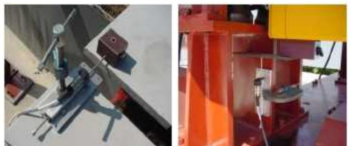
Figure9. Installation of measuring instrument for a thermal expansion about longitudinal and vertical directions
