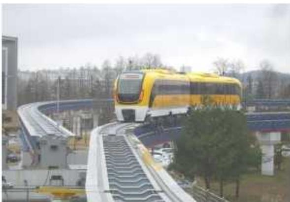
Figure7. Maglev vehicle running on the segmented switch
