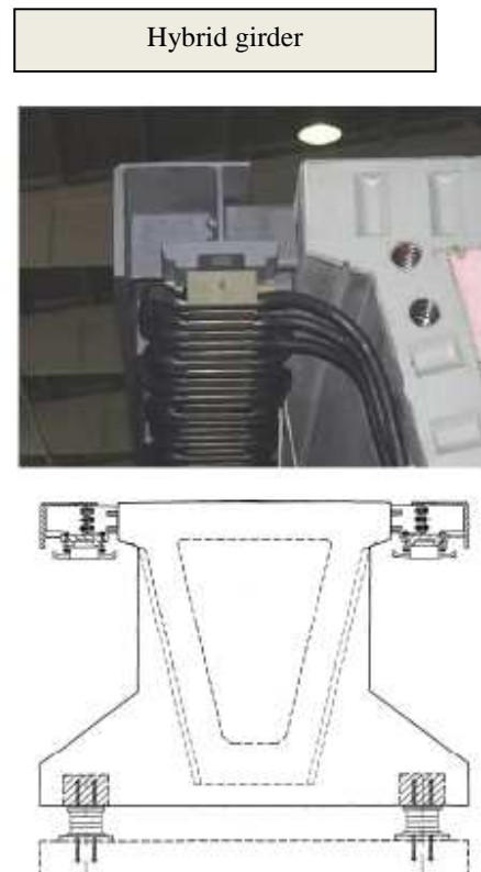
Figure 4: Hybrid girder (Shanghai) functional level and cross-section
