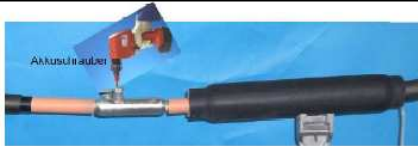
Figure 11: System of connecting cables at side
