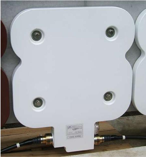
Figure 5. Photo of ground coil type of PLG
