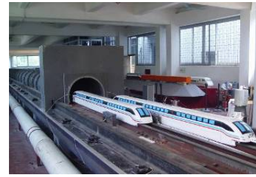
Figure 3 the model test of maglev tunnel
