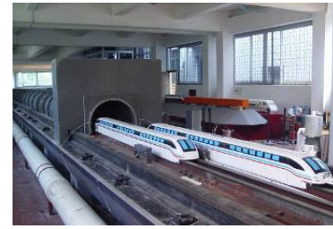
Figure 3 the model test of maglev tunnel
