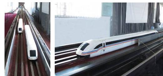
Figure 15 model test for aerodynamic effect
