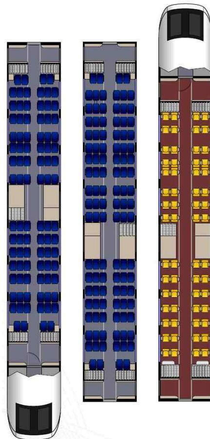
Figure 8. Seating arrangements of the SMT Shanghai Transrapid as an example of short and regional-distance transportation [8].
