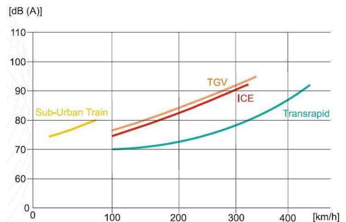
Figure 6. Maglev trains are always quieter in comparison to traditional systems when operating at the same speeds [8].
