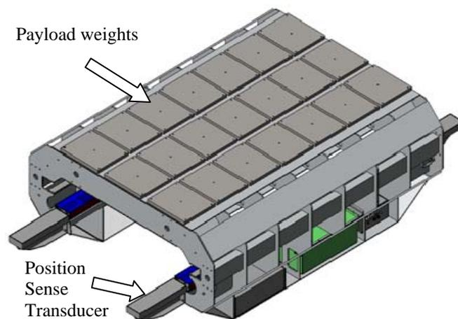
Figure 2. Isometric view of Test Sled
