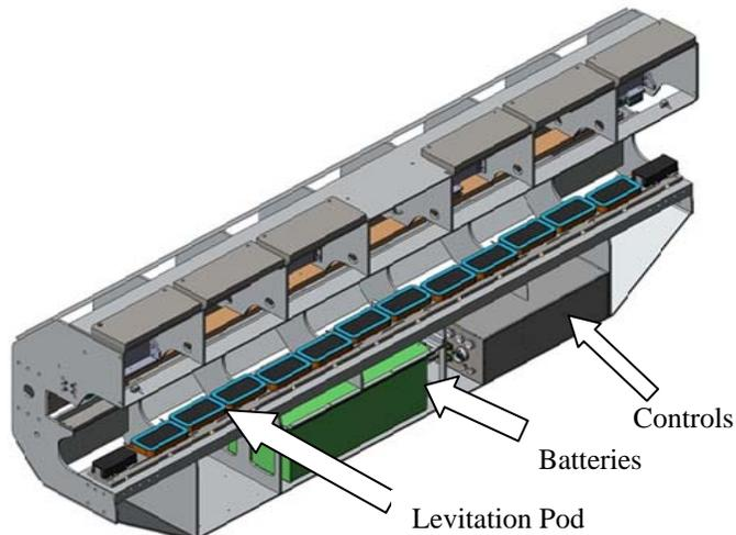
Figure 1. Levitation array and electronics locations
