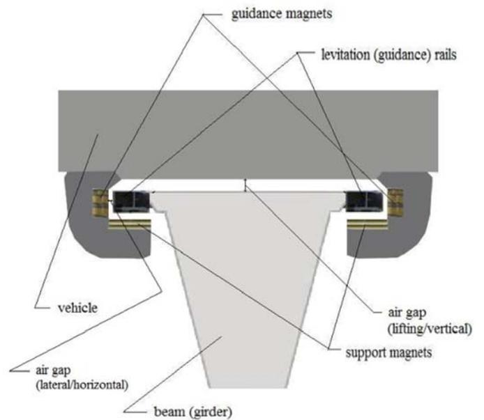
Figure 2. Caption schematic diagram of EMS maglev system.
