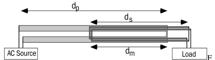
Figure 7. Inductive power transfer module.
