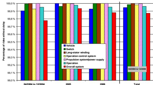
Figure 2. Annual punctuality of the Shanghai Transrapid, delays of more than 5 min
