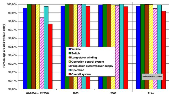
Figure 3. Annual punctuality of the Shanghai Transrapid, delays from 20 s to 2 min
