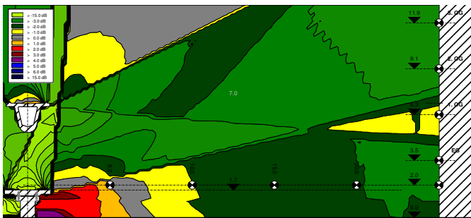
Figure 8 Differences of the acoustic emissions for guideways on stilts and guideways at ground level
