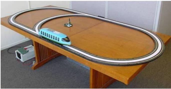
Figure 5. Sub-scale SPM Maglev test track
