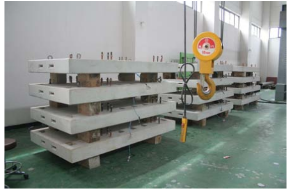
Figure 10. Stack of 2.5m rectangular precast deck
