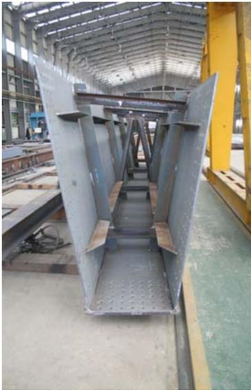
Figure 13. Section view of trapezoidal open steel box girder
