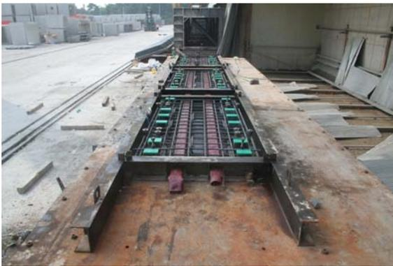
Figure 8. 3 Steel forms and arrangement of reinforcement bar
