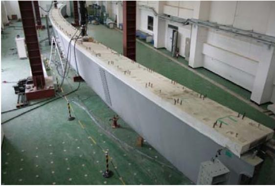
Figure 18. Overview of integration of trapezoidal open steel box girder and precast decks
