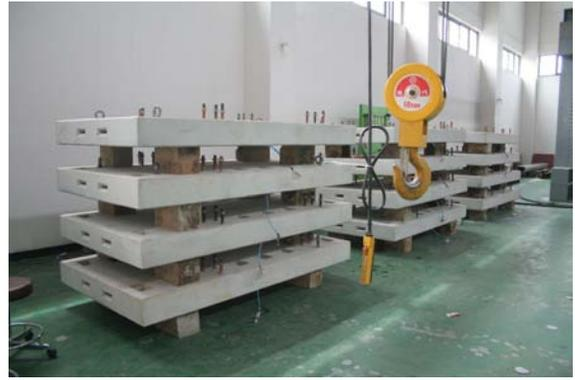
Figure 10. Stack of 2.5m rectangular precast deck
