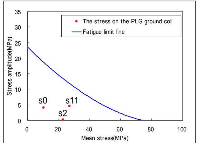
Figure 12 the stress limit diagram of molded resin
