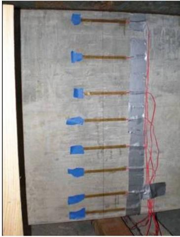
Figure 5. Test beam strain gages.
