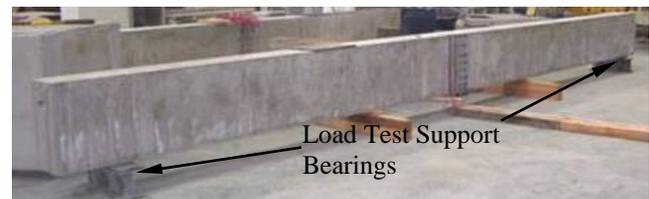
Figure 3. Quarter-scale non post-tensioned static load test beam.
