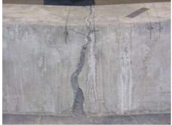
Figure 6. Test beam brittle fracture.
