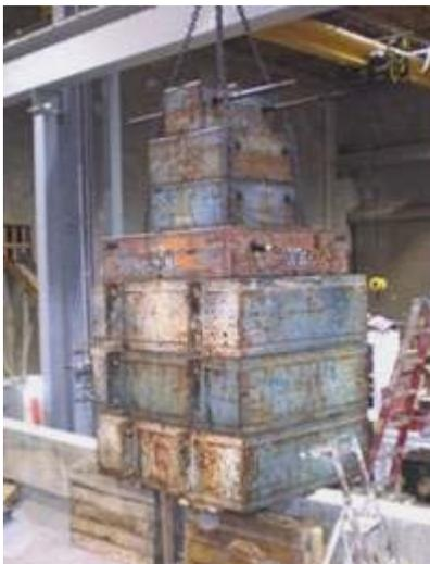
Figure 4. Post-tensioned beam supporting 81,250 lb load.
