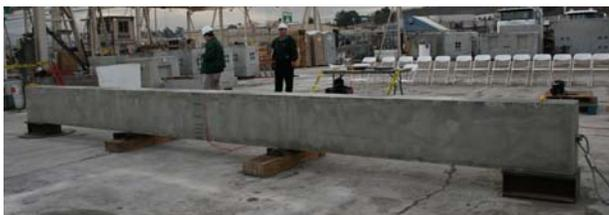
Figure 1. Quarter-scale post-tensioned static load test beam.
