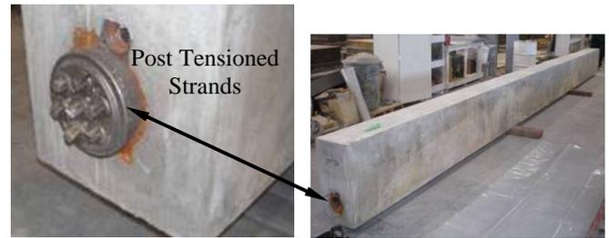
Figure 2. Quarter-scale post-tensioned static load test beam.
