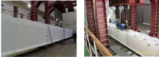
Figure 6. Static and vibration test
