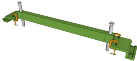
Figure 10. Temporary rail support jig
