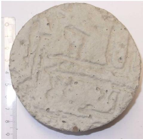
Figure 3. Specimen prepared with form liner.
