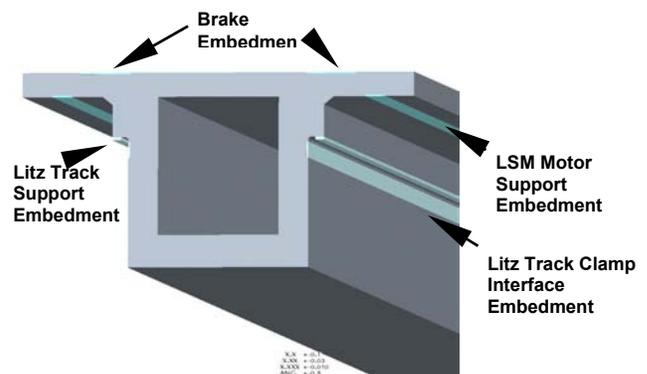
Figure 2. IGGM girder with embedded features
