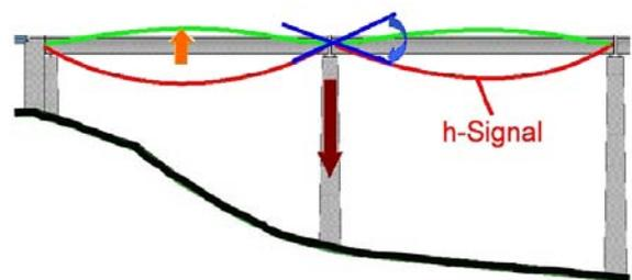
Figure 3: Parameter of „long wave“ guideway contour
