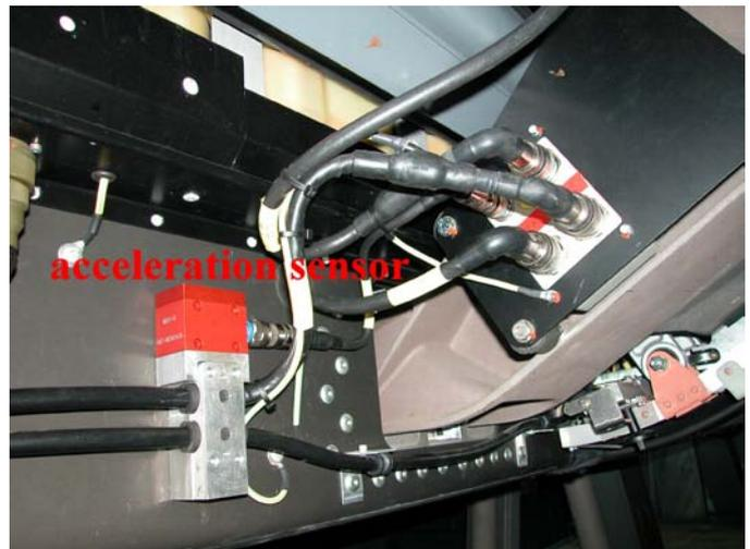
Figure 7: acceleration sensor at the levitation magnet
