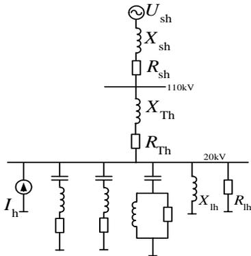
Fig.1 The schematic diagram of the filter
