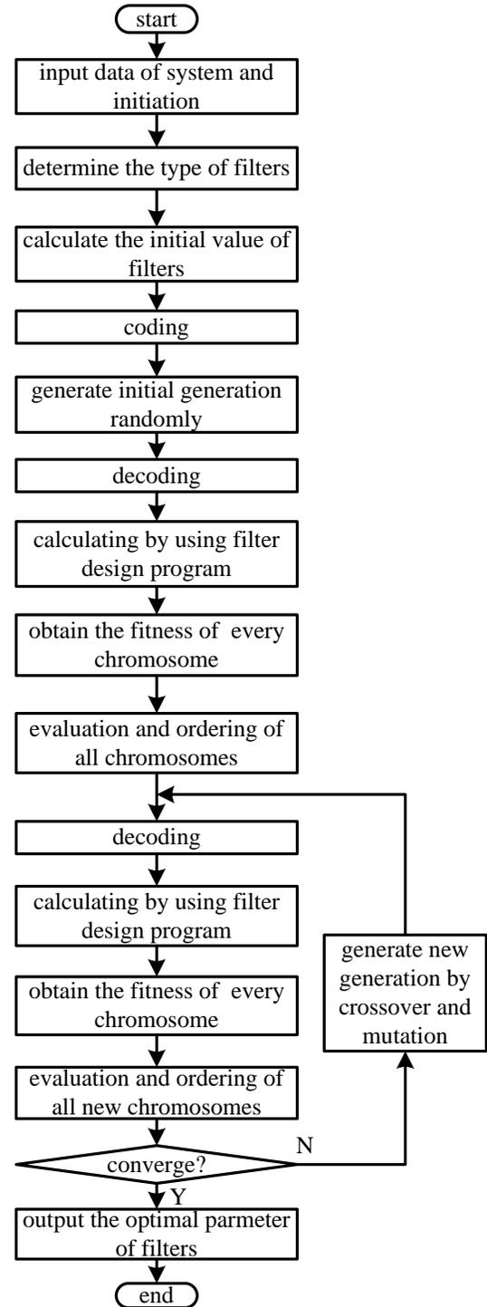
Fig.4 Flowchart of the optimal parameters of filter system using IGA
