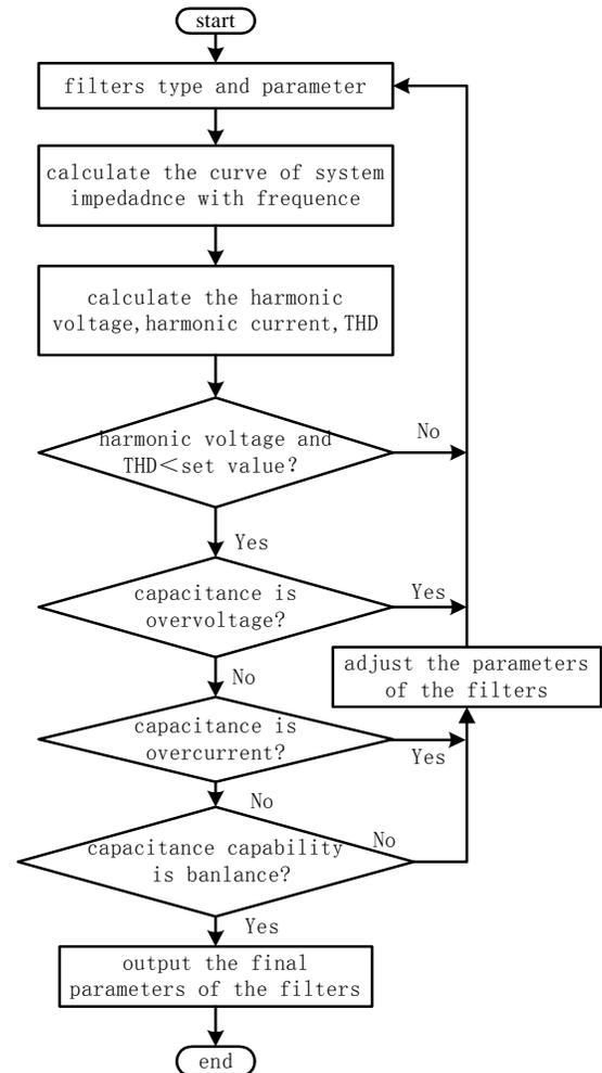
Fig.2 Flow chart of the filter system design
