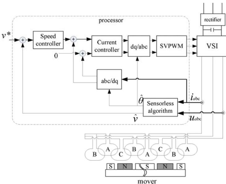
Figure 1. Sensorless vector control of LSLSM.
