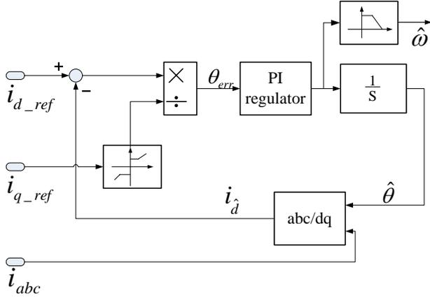
Figure 3. Sensorless scheme diagram.
