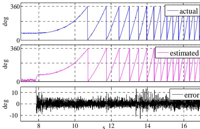
Figure 6. Mover position estimation. (a) actual position; (b) estimated position; (c) estimation error.
