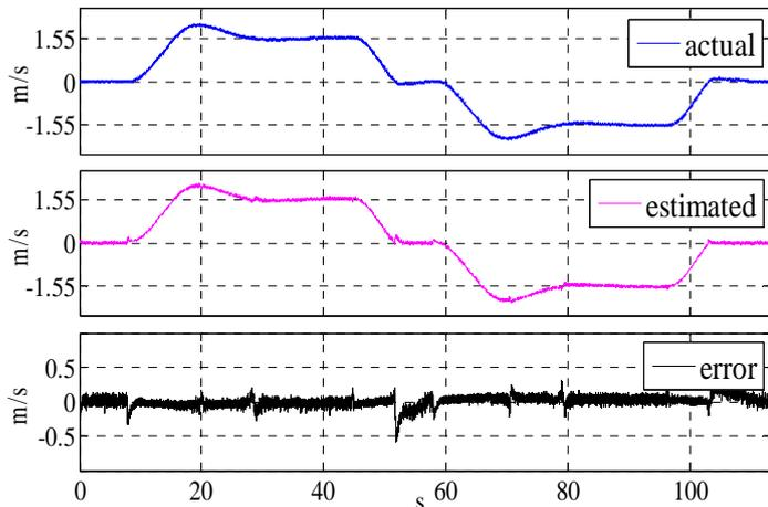
Figure 5. Mover speed estimation. (a) actual speed; (b) estimated speed; (c) estimation error.
