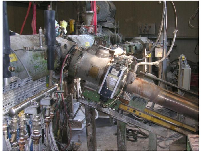
Figure 5: CV line used for manufacturing the outer sheath
