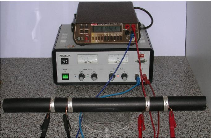
Figure 7: Test set-up for electrical resistance measurement
