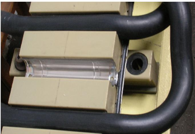
Figure 3: Grounding steel jacket with clamp on the right side. In this picture, the earthing rope is sheathed with a semi-conductive material
