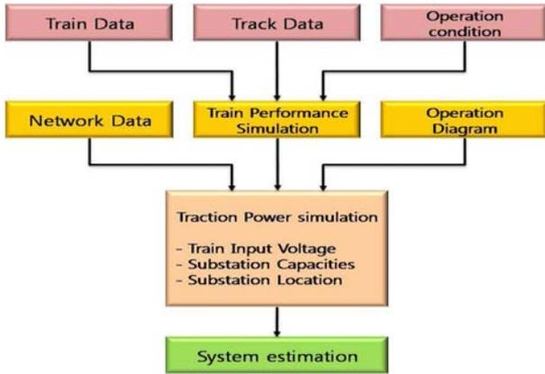
Figure 4. Traction power system simulation structure.
