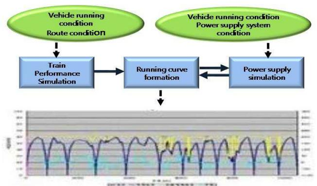
Figure 1. Diagram on execution of traction power supply simulation.
