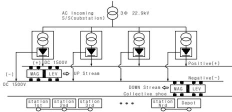
Figure 2. DC-fed traction power system.
