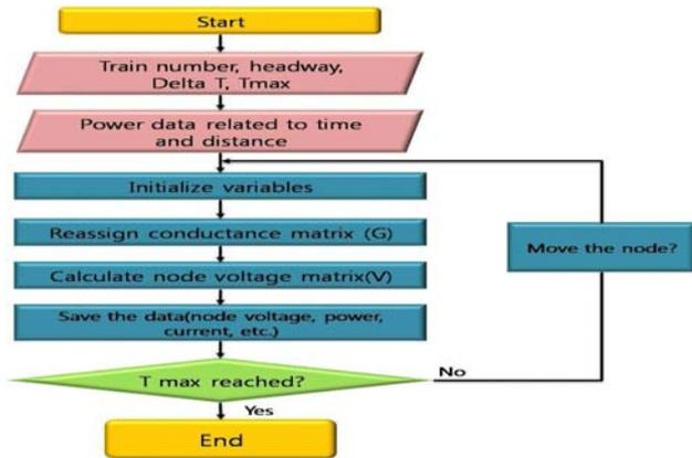
Figure 5. Simulation algorithm flowchart.
