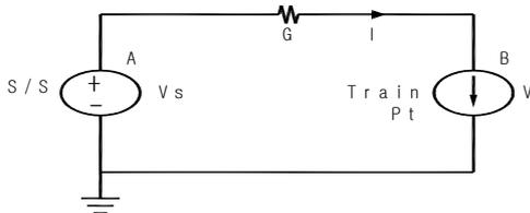
shown schematically for power analysis in Fig.3. The DC voltage source,  $V_s$ , feeds a train load which draws power  $P_t$  through the conductor rail with conductance  $G$ .
