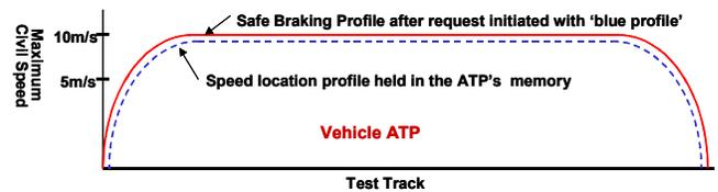
The onboard ATP has the maximum civil speed profile in its memory. If at any time the vehicle violates the threshold profile (blue), emergency braking is requested and the inverter is requested to be shut off.
