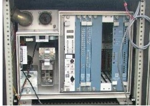
Figure 8: Vehicle onboard ATP rack.
