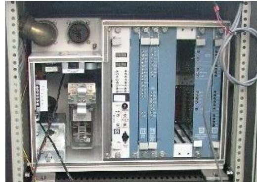
Figure 8: Vehicle onboard ATP rack.
