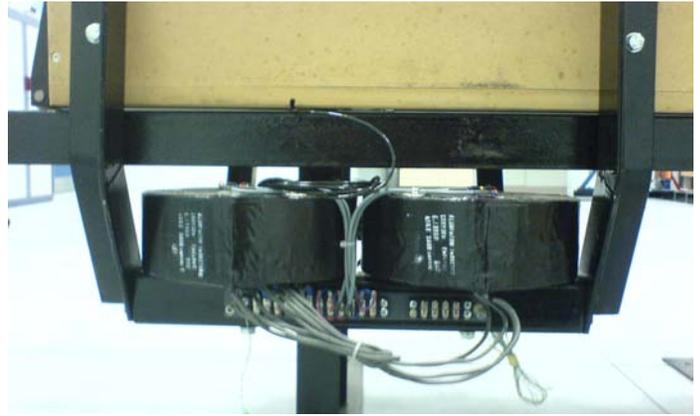
Figure 4: Photo of magnet with dual wound coils
