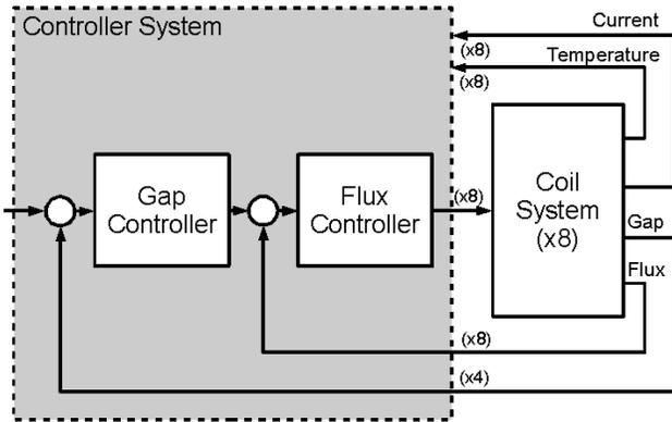
Figure 6: Control structure of Maglev test rig
