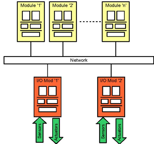
Figure 2: Concept network of IMS modules
