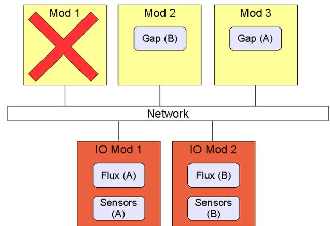
Figure 11: Example of Reconfiguration
