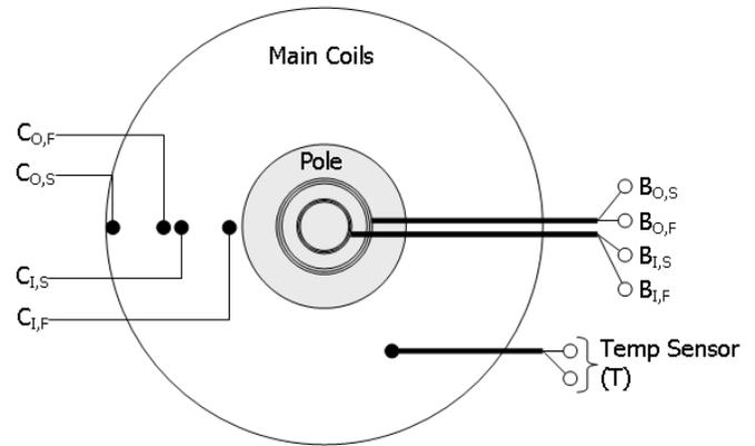
Figure 5: Schematic of coil windings
