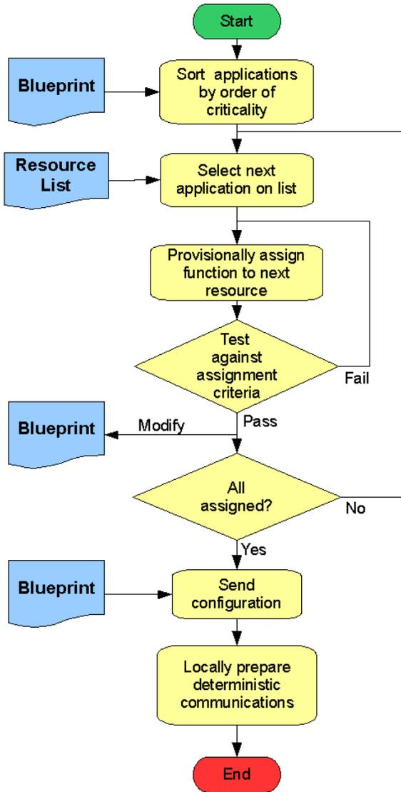
Figure 8: Flow diagram of system configuration
