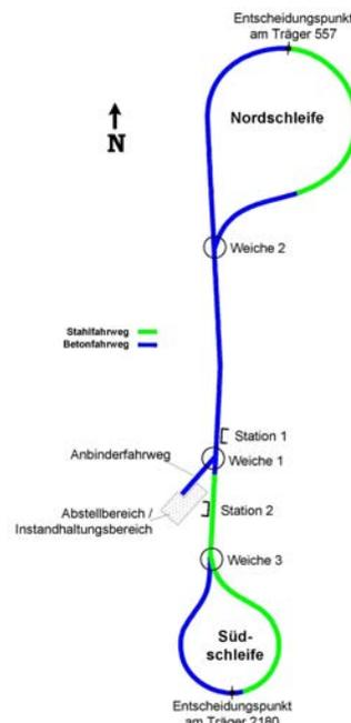
Figure 1: Transrapid test facility: Track layout
