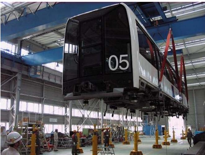
Figure 3. Separation of body and modules
