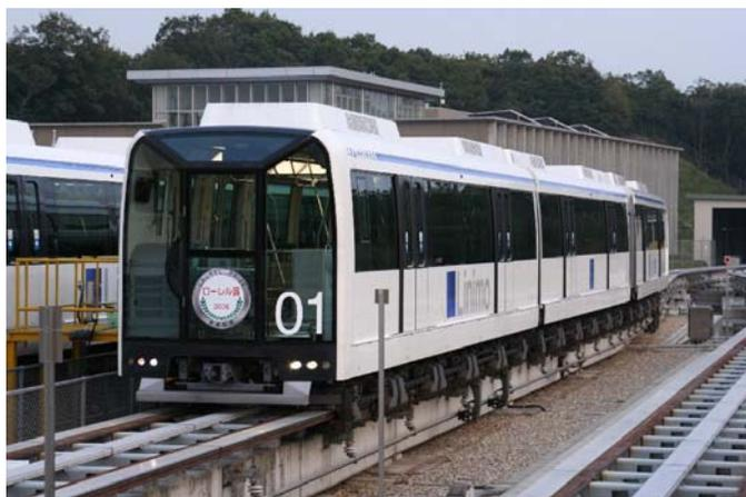
Figure 1. HSST vehicle (Linimo vehicle)
