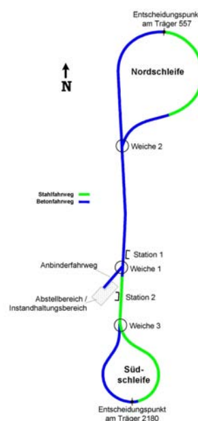
Figure 1: Transrapid test facility: Track layout
