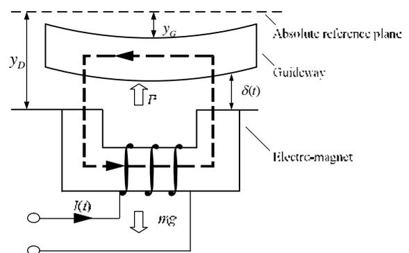
Figure 1. Schematic of mono-electromagnet magnetic levitation system in absolute reference plane
