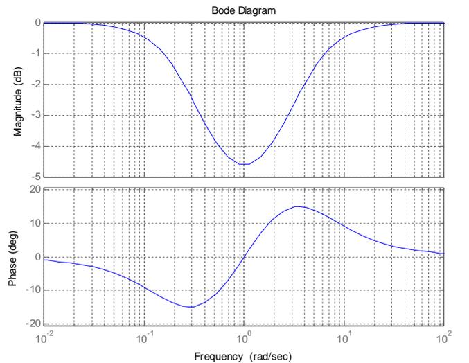
Figure 2. Example of bode plot of band-stop filter
