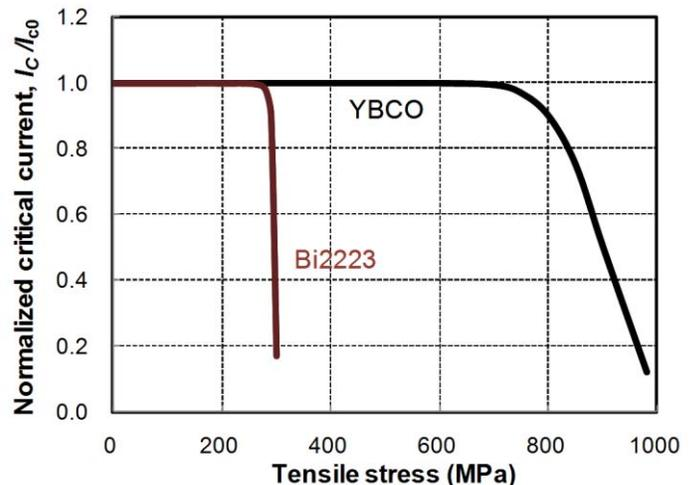
Figure 3. Tensile stress dependence of normalized  $I_C$  (Example data).
