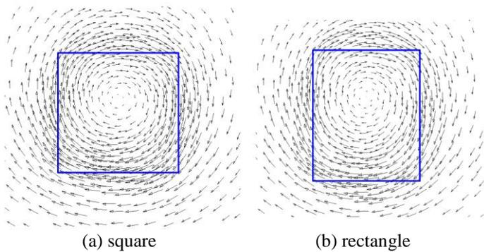
Figure 7. Dependence of magnetic fields on the shape of coil cross section.
