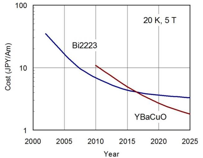
Figure 2. Cost projection of Bi2223 and YBCO wires.
