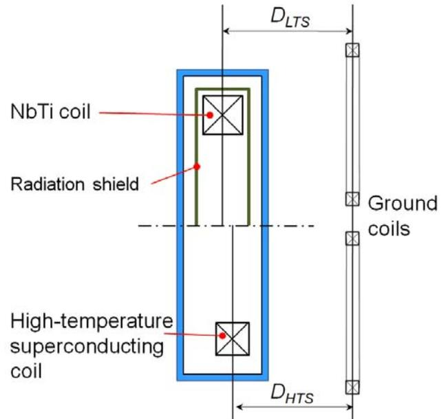
Figure 5. Reduced distance between a superconducting coil and a ground coil ( $D_{HTS} < D_{LTS}$ ).
