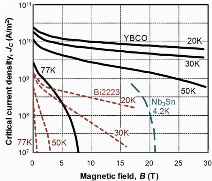
Figure 1. Performance of high-temperature superconductors ( $J_C$ - $B$ - $T$  characteristics).
