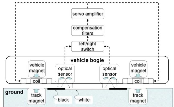
Figure 6. The elements of the lateral stabilization loop.
