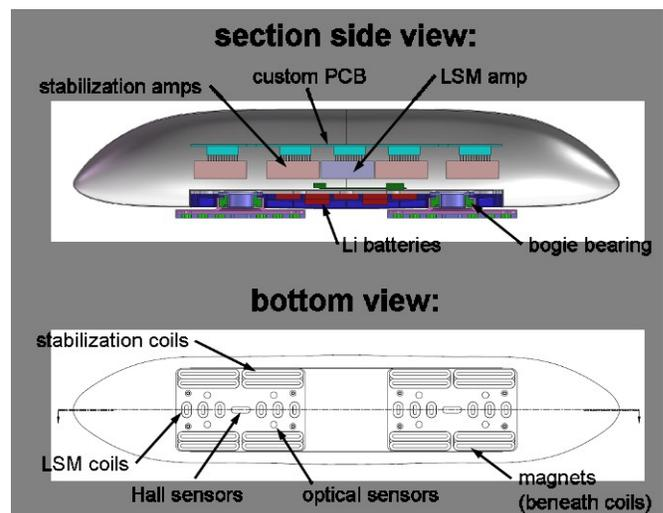
Figure 4. Two views showing several key components.
