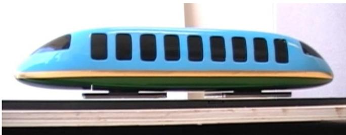
Figure 2. top: The prototype on its track; bottom: A close-up view of the small-scale prototype vehicle levitating.
