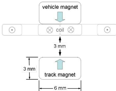
Figure 5. The track and vehicle magnet configuration.
