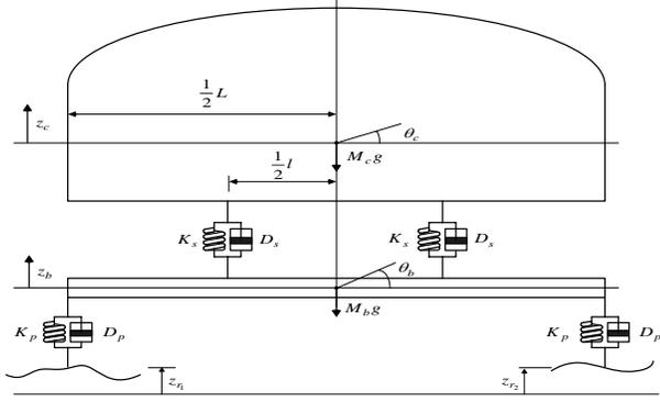
Figure 9. Simplified maglev vehicle and second suspension
