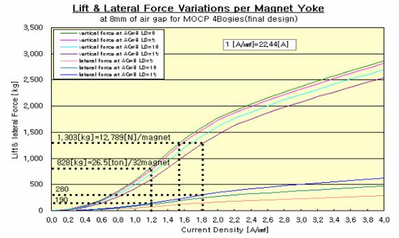
Figure 1. Levitation & guidance force at nominal air gap(8mm)
