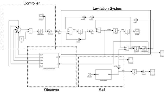
Figure 12. Block diagram for the single magnet control system.
