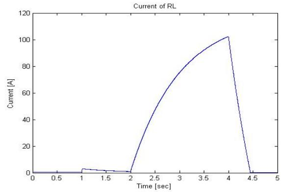
Figure 6. Load current profile by using dual chopper
