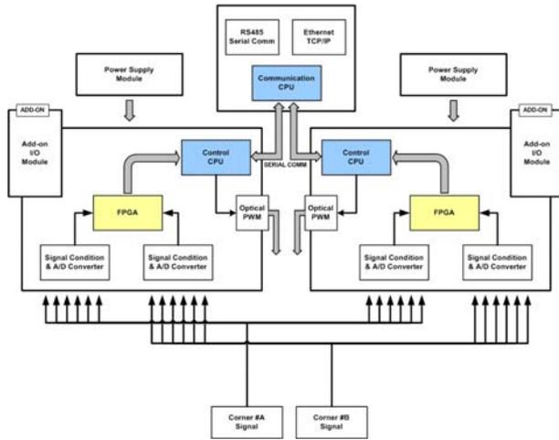
Figure 4. Structure of the controller unit.
