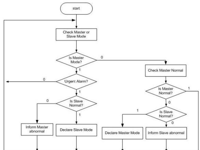
Figure 8. Flowchart of switch from master mode to slave mode
