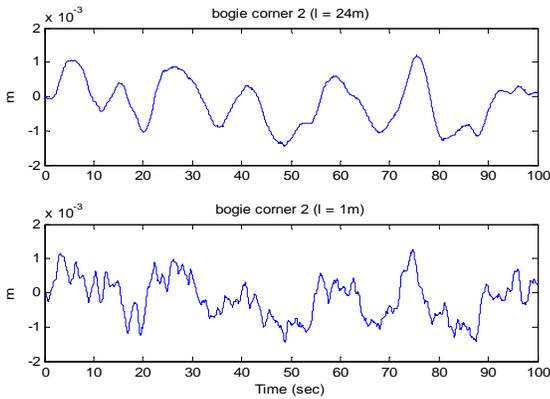
Figure 10. Profiles of bogie corner according to second suspension position.
