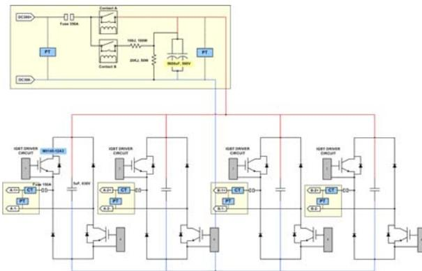
Figure 5. Structure of the chopper unit.
