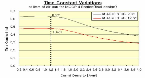
Figure 2. time constant to current density and temperature
