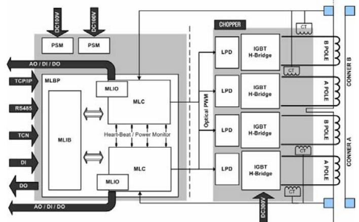
Figure 3. Structure of the magnet driver
