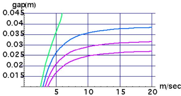
Figure 3: Plots of the gap as a function of velocity for loads of 240 kN (lowest curve), 220 kN, 200 kN, and 180 kN.
