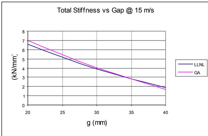
Figure 10: Total stiffness of 5 x 3 array plus LSM system vs. levitation gap for velocity of 15 m/sec.
