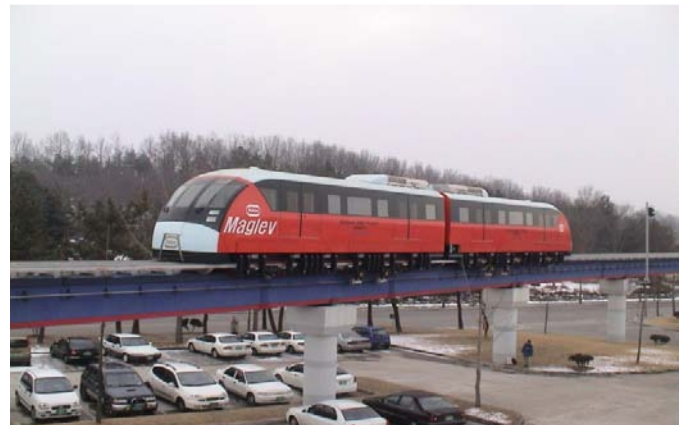
Figure 4. Urban maglev vehicle UTM-02 running over a flexible guideway.
