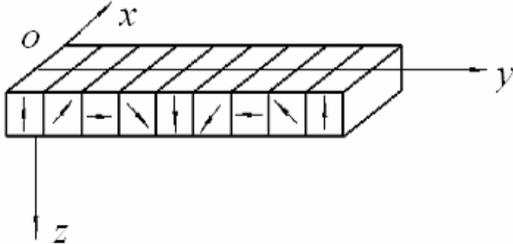
Fig 2 Halbach array and the coordinate system
