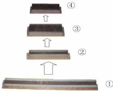
Fig10 Four Halbach arrays made in the lab
