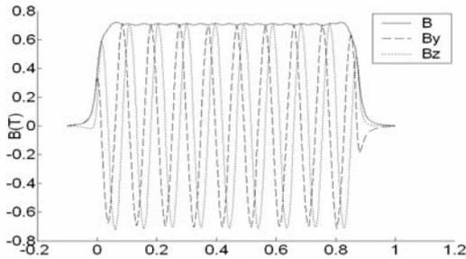
Fig 9 Magnetic field of offset-Halbach array
