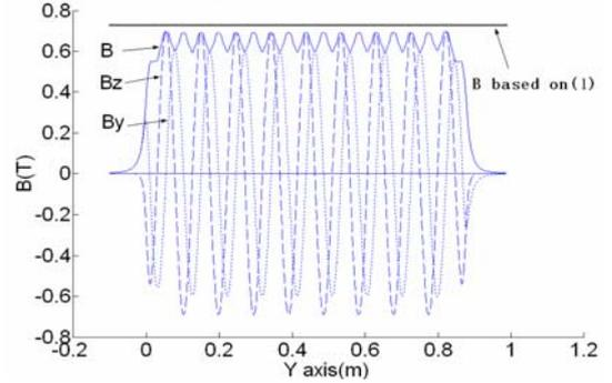
Fig 3 Fields of linear Halbach array based on magnetization charges
