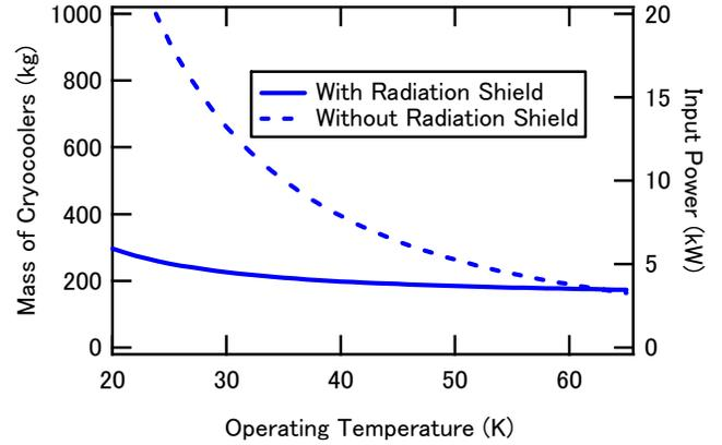
Figure 5. Estimated mass and input power of cryocoolers as a function of the operating temperature.
