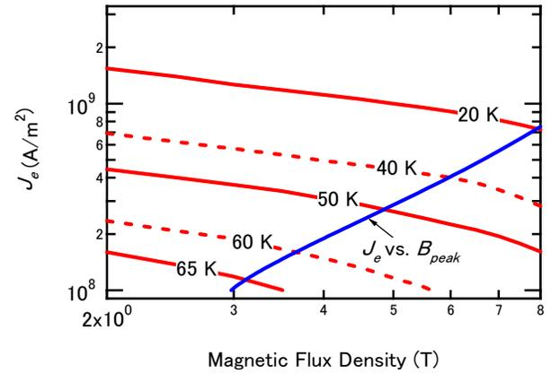
Figure 2. Estimated  $J_e$  characteristics of 2G wire and the calculated  $J_e-B_{peak}$  line of the racetrack coil. The crossings of  $J_e-B$  curves and the  $J_e-B_{peak}$  curve indicate design points of the coil at each operating temperature.
