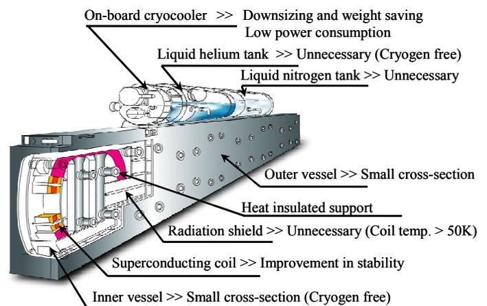
Figure 1. Merits of applying 2G wires to a superconducting magnet for the maglev train. The original figure is a schematic view of a superconducting magnet with Nb-Ti coils.
