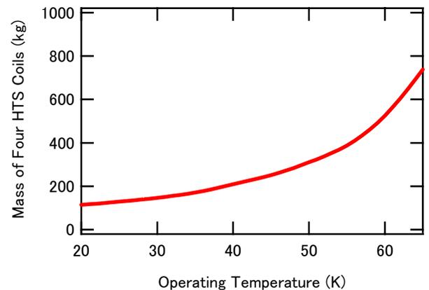
Figure 3. Estimated mass of four HTS coils as a function of the operating temperature.
