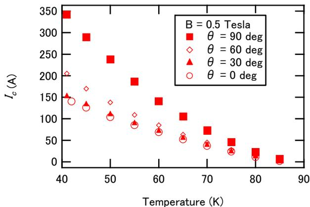
Figure 7. Measured  $I_c$  characteristics of 2G wire sample at various operating temperatures and applied magnetic field directions  $\theta$ .
