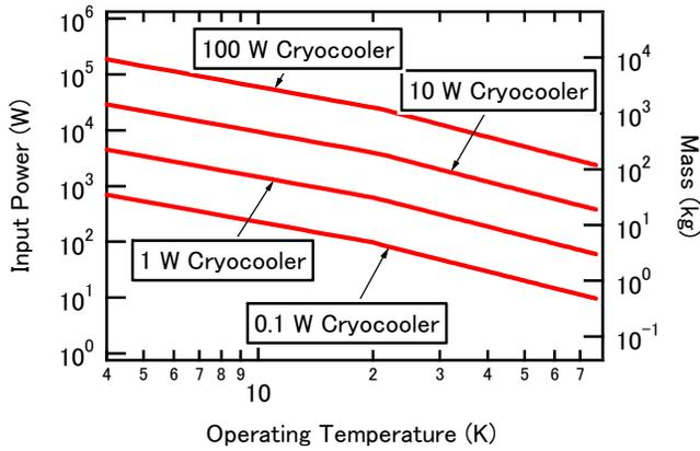
Figure 4. Plot of the mass and power consumption of cryocoolers operating at various temperatures and cooling capacities.
