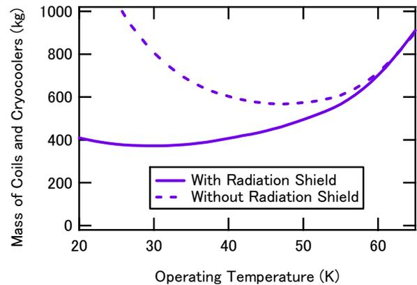
Figure 6. Estimated mass of four superconducting coils and cryocoolers as a function of the operating temperature.
