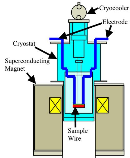
Figure 8. Schematic diagram of the system for measuring the properties of 2G wires.
