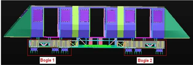
Figure 3. FE model of the Vehicle with 2 bogies
