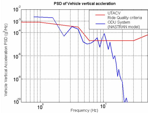
Figure 14. PSD of vehicle vertical acceleration of ODU system
