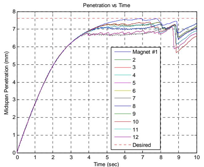
Figure 11. Actual air gap of 12 magnets
