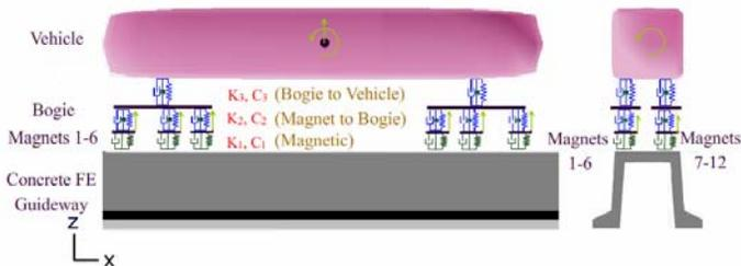
Figure 5. A 21 DOF Dynamic model of ODU system
