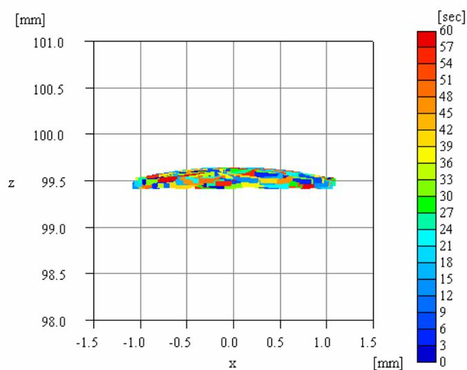
(a) Trajectory of the PM center of a top started at (1, 0, 99.5)
