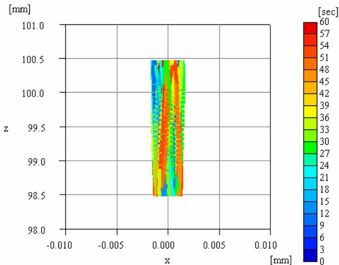
(b) Trajectory of the PM center of a top started at (0, 0, 98.5)
