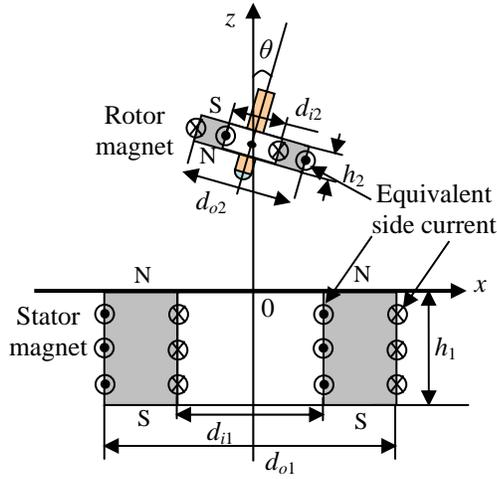
Figure 2. Analytical Model of The Magnetic Top
