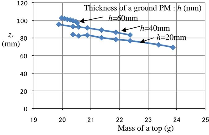
Figure 4. Height of the restoring center v.s. mass of levitating top.
