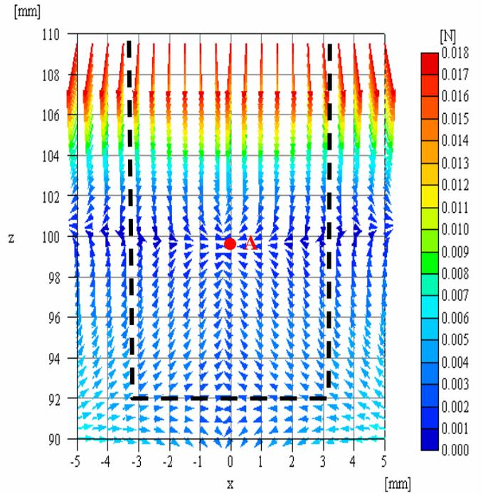
Figure 3. Levitating area and restoring center in the force map.
