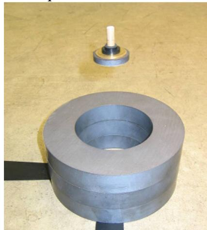
Figure 1. Levitating magnetic top.
