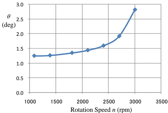
Figure 7. The maximum tilt angle  $\theta$  v.s. rotating speed.
