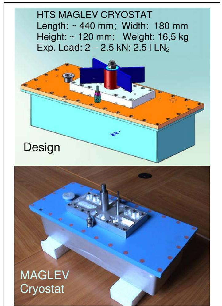
Figure 9 Design and assembled HTS MAGLEV cryostat.
