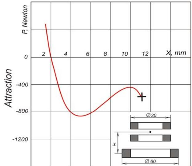
Figure 6. MPW-suspension nearby the critical current mode.
