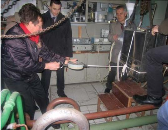
Figure 10. MPW-force measurements by hand.
