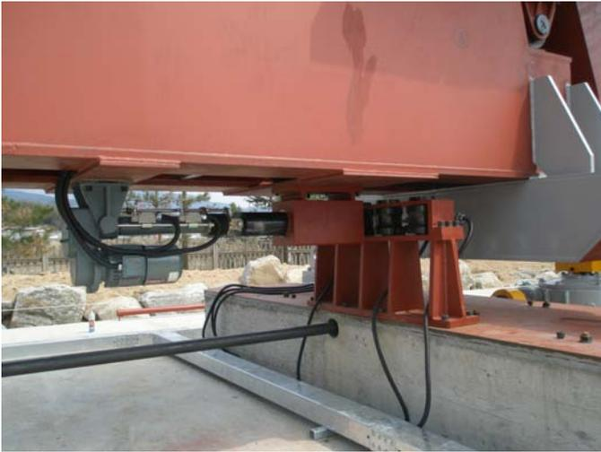
Figure 7. Switch locking device
