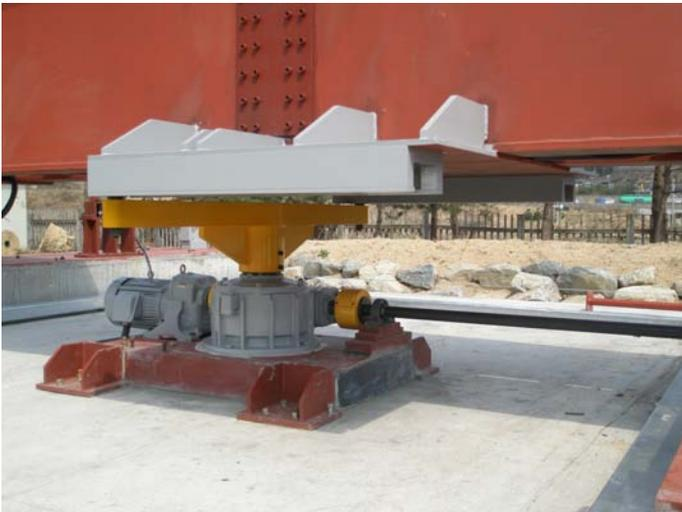
Figure 8. Main switch driving motor, gear reducer, and the rotating arm
