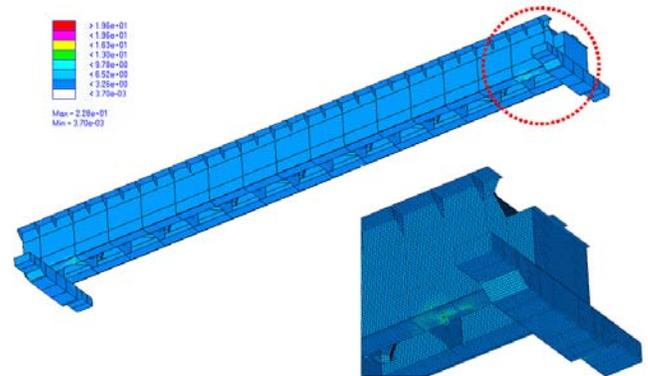
Figure 3. Stress Distribution of the No. 3 switch girder
