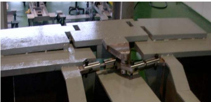
Figure 9. Articulation angle halving link
