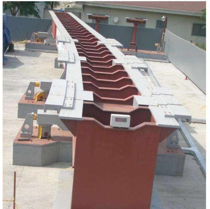
Figure 6. 3 way segmented switch aligned at turn out
