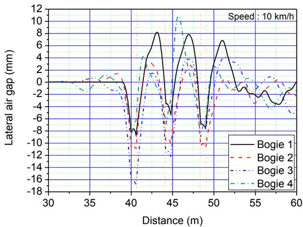
Figure 4. Lateral air gap deviation as the train proceeds in the switch turn out direction. Train speed  $V = 10$  km/h
