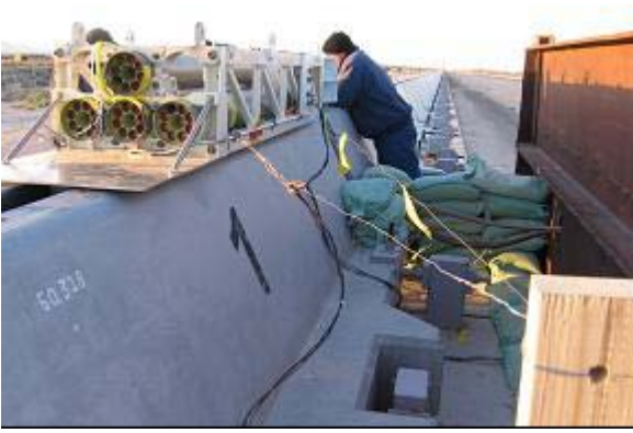
Figure 11. Sled with 4 HVAR motors installed
