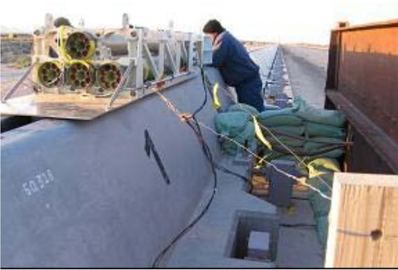
Figure 11. Sled with 4 HVAR motors installed
