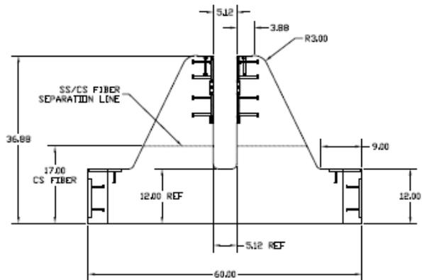
Figure 6. Guideway crosssection view (dimension in inch)
