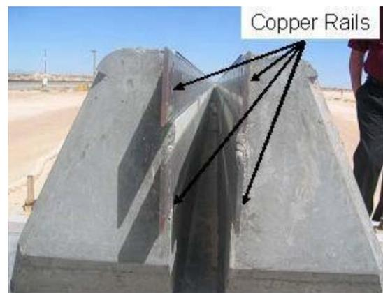
Figure 7. Copper rail embedded in the concrete guideway
