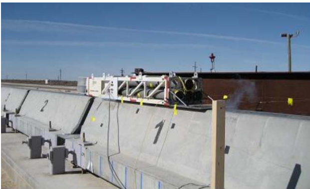
Figure 12. Rocket sled with 4 HVAR motors ready for flight test
