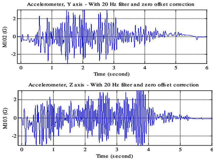
Figure 17. Accelerometer data in heave and sway directions
