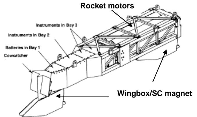
Figure 3. Sled with wingboxes mounted and motors loaded
