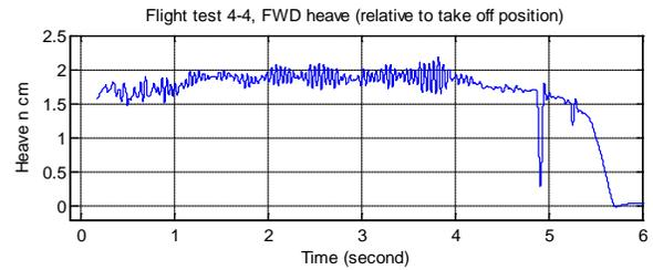
Figure 14. Sled position (relative to take off) versus time
