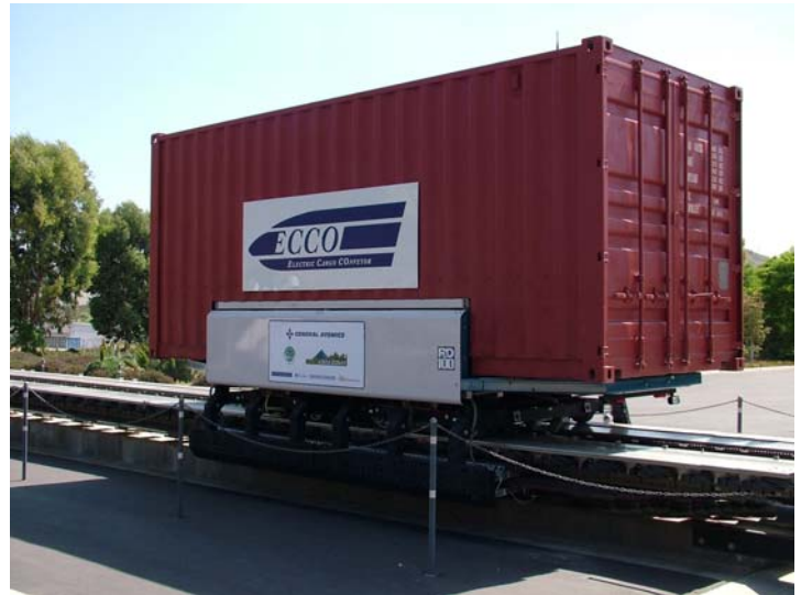
Figure 3. World's First Maglev Container Move at General Atomics San Diego, CA, June 2006.
