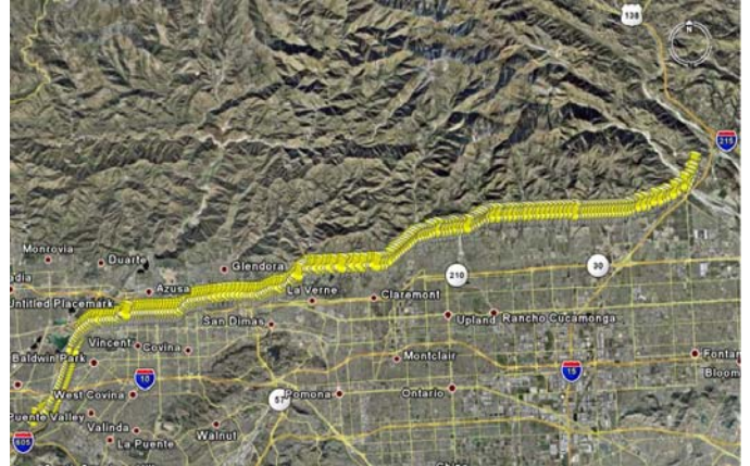
Figure 7. DC Transmission Line Route from Downtown LA to the Foot of the El Cajon Pass
