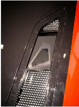
Figure 11. Camera system integrated in the front lights
