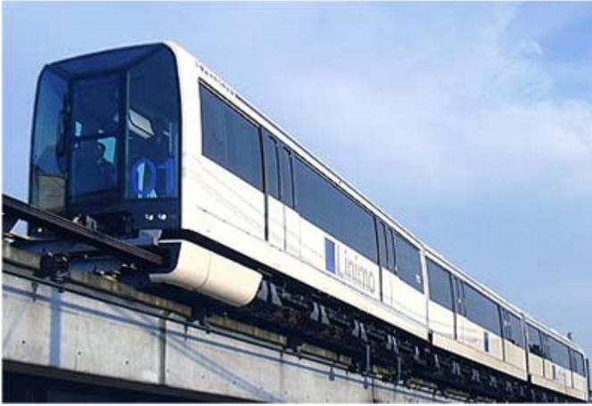
Figure 4. Picture of the Japanese, low-speed, EMS-type MagLev train on the Linimo line.
