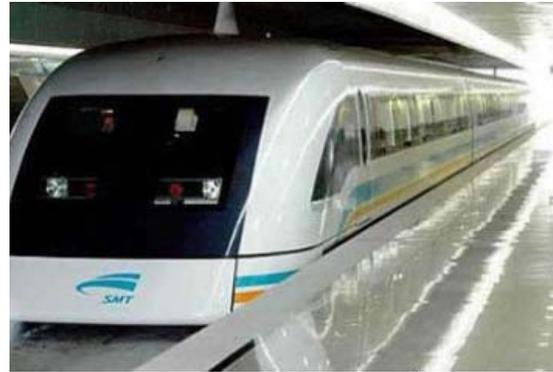
Figure 2. The high-speed, Chinese-Transrapid EMS-type MagLev train.
