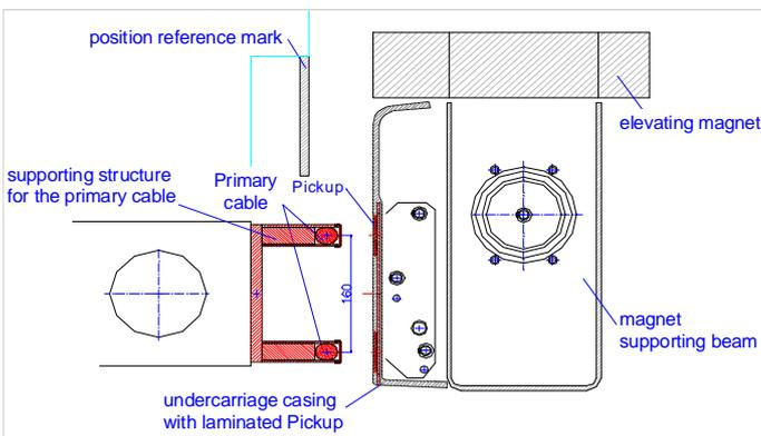
Figure 8. Detail of the IPS system (Source: ThyssenKrupp)
