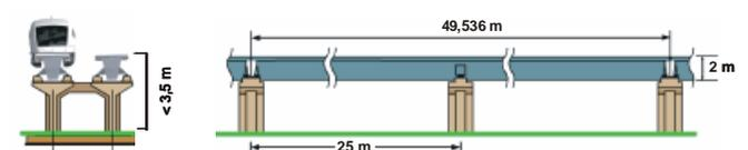
Figure 6. Types of Maglev Guideway Beams
