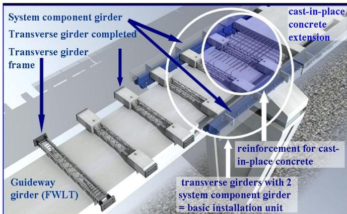
Figure 4. Track of Type II, BGmU design (Source: BGmU)
