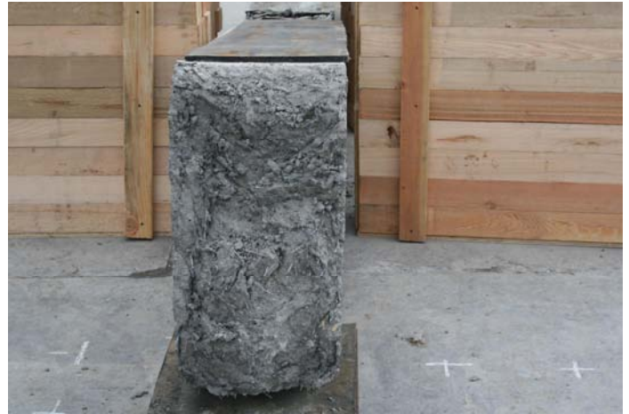
Figure 9. Failed Hybrid Test Beam Due to Brittle Fracture
