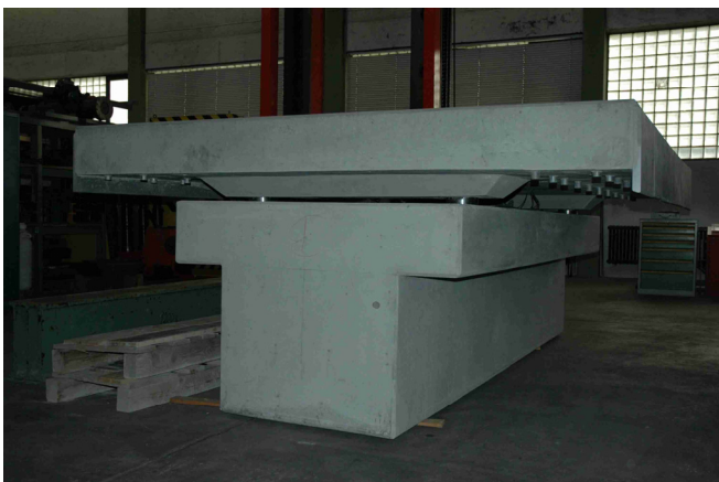
Picture 1: First test set-up of the new guideway
