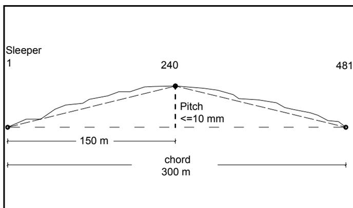
Figure 6: Wheel-on-rail - Internal, long-wave deviation for the determination of periodic effects
