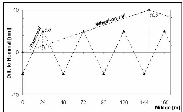
Figure 9: Comparison of the long-wave tolerances
