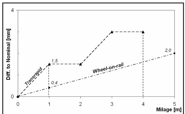
Figure 7: Comparison of change of inclination criterion and internal shortwave geometry
