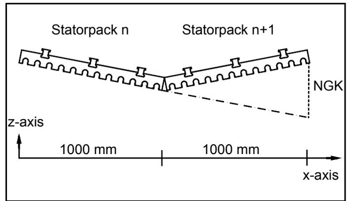
Figure 4: Transrapid: Change of inclination criteria at the the stator plane
