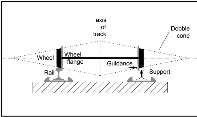
Figure 2: Support and Guidance at wheel-on-rail
