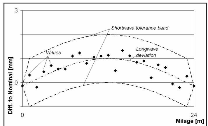
Figure 3: Transrapid – one-span-girder: longwave and shortwave deviation
