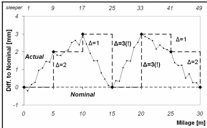
Figure 5: Wheel-on-rail - Internal, shortwave deviation for the determination of single deviation
