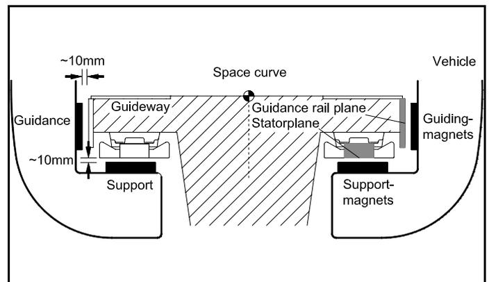
Figure 1: Support and guidance at the Transrapid
