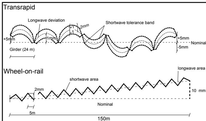
Figure 8: Comparison of the internal geometry by means of tolerance ranges
