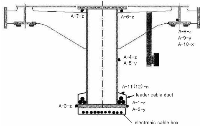
Figure 2: Test positions layout on the guideway switch
